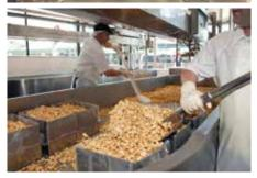
(Top to bottom) After the cheesemaker has cut the curds to release the whey, the curds are cut again and stacked into loaves. The loaves are then run through a curd cutting mill, creating uniform curds that are scooped into hoops before being set aside for aging.
